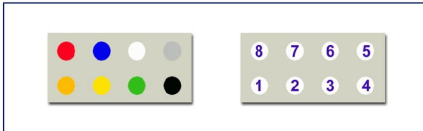
To make it easier for you to correctly insert the plug first time, manufacturers will usually mark the #1 or Orange pin with an asterisk, a star or the number 1. Look carefully... it's not always obvious!
