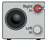
Leave 'Left' RCA jack disconnected. Wrap in electrical tape to prevent short circuit.
