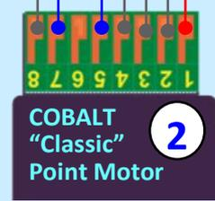
Properly interlocked LEDs have been achieved just by using their polarity and control of LED power via Cobalt number 2. This still leaves us a completely "free switch" on Cobalt # 1 !
