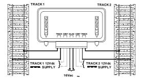
Disconnect any previously fitted track supplies. Connect the unit as shown in the diagram. Without a locomotive on the tracks the neon indicators will glow and it may be possible to detect a tingling sensation when touching the track. Placing a locomotive on the track will cause the relevant neon indicator to extinguish.
