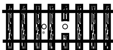
Remove or cut one sleeper as shown, then drill two 3.5mm holes 11mm apart and counter-sink the one marked with \*.
