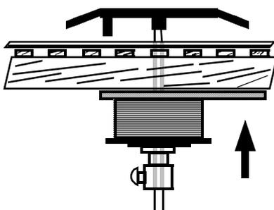
Loosen grub screw and disassemble the unit. Then reassemble in position as shown. Use a screw through hole indicated by arrow for fixing.
