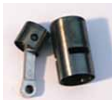
PAW 15GTS engine parts showed very little carbon after test
